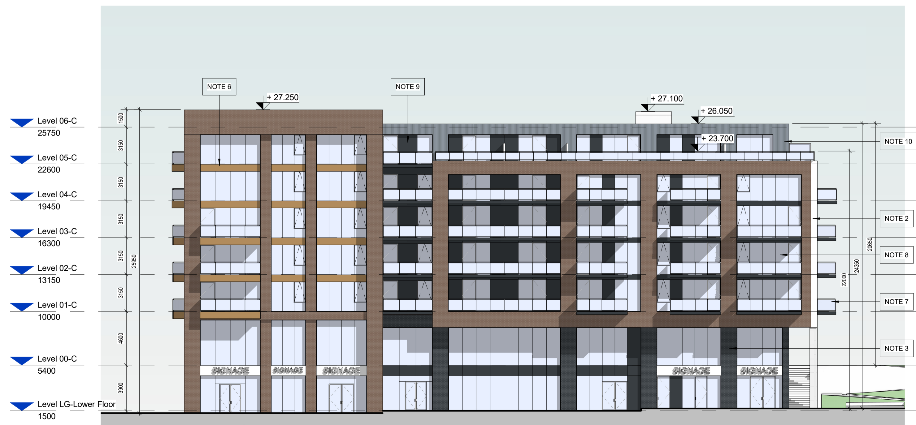
2 BLOCK C-SOUTH ELEVATION 1 : 200
